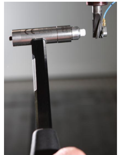
"Tap-test" of a milling tool – part of the vibration analysis.
